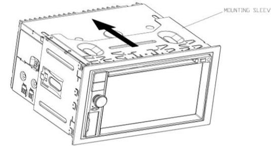
With the sleeve fully inserted into the dashboard opening, bend as many of the tabs outward as necessary to firmly secure the sleeve to the dashboard.
