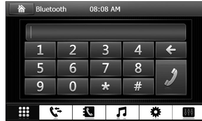
2. Using the keypad, touch 0-9, \*, #, to enter the phone number you wish to dial. If you enter an incorrect number, touch the icon on the keypad to delete the incorrect number.
