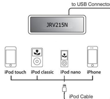
**NOTE: The iPod will continuously recharge when connected to the unit, as long as the vehicle ignition is turned on.**
