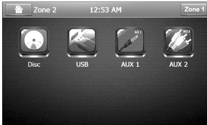
The Zone 2 function allows the radio to operate two different modes concurrently, one for the driver, and one for the passengers. For example, the driver is able to listening to the radio while the passengers are watching a DVD. There is no interference between Zone 1 and Zone 2.
